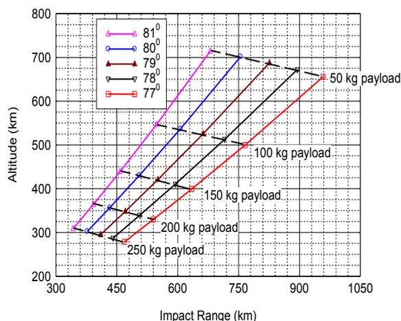
**Fig.9. Performance of sounding rocket for various LEA with different payloads**
