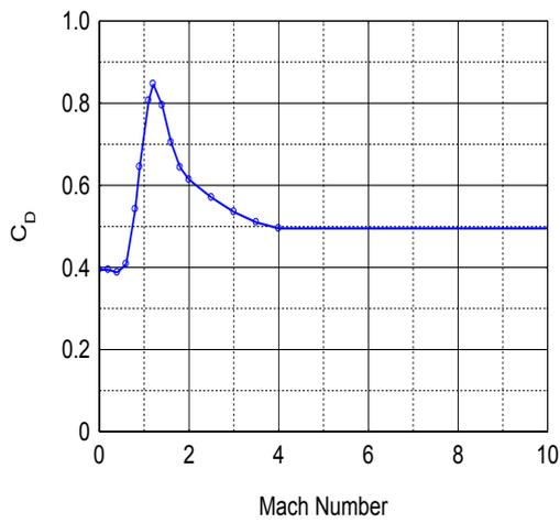
Fig.2. Drag Coefficient with respect to Mach No.
