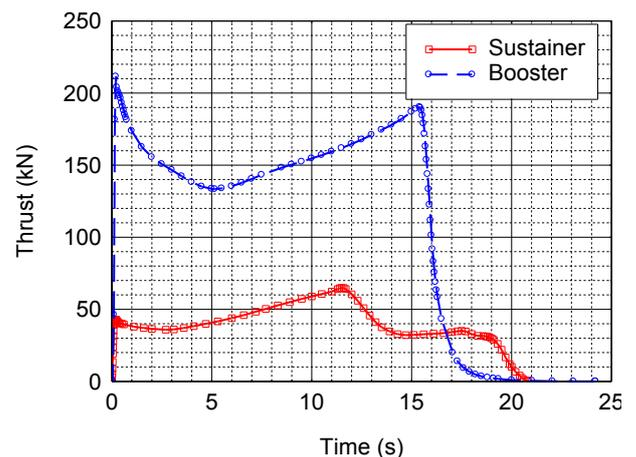
**Fig.1. Thrust-Time Profile of the Rocket**
