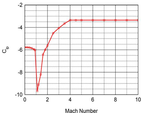
Fig.5. Dynamic Derivative (Roll damping moment coefficient derivative due to rolling velocity) Vs Mach No.
