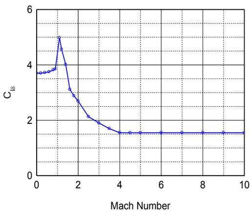
Fig.4. Rolling moment coefficient derivative due to booster fin cant Vs Mach No.
