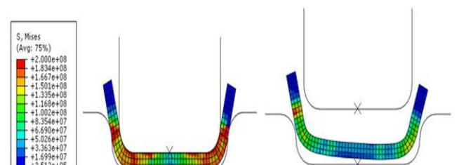
**Fig.7:** Stress fields for 4 mm corner radius (Stress in Pascal). (a) Stress mapping during maximum deep-drawing, (b) deformation of the sheet metal after the deep-drawing operation
