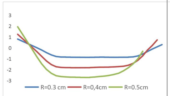
**Fig.9:** Comparison of the residual deformations of the sheet metal after the deep-drawing operation for different corner radius
