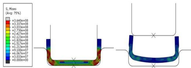
**Fig.6:** Stress fields for 2.5 mm corner radius (Stress in Pascal). (a) Stress mapping during maximum deep-drawing, (b) deformation of the sheet metal after the deep-drawing operation.
