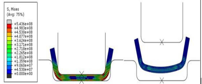
**Fig.3:** Stress fields for a 0.35mm gap between the sheet metal and the punch (Stress in Pascal). (a) Stress mapping during maximum deep-drawing, (b) deformation of the sheet metal after the deep-drawing operation
