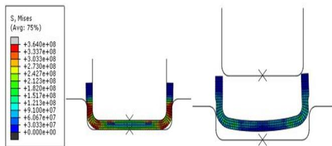
**Fig.2:** Stress fields for a 0.25mm gap between the sheet metal and the punch (Stress in Pascal). (a) Stress mapping during maximum deep-drawing, (b) deformation of the sheet metal after the deep-drawing operation.
