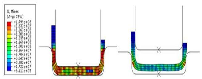
**Fig.8:** Stress fields for 5 mm corner radius (Stress in Pascal). (a) Stress mapping during maximum deep-drawing, (b) deformation of the sheet metal after the deep-drawing operation.
