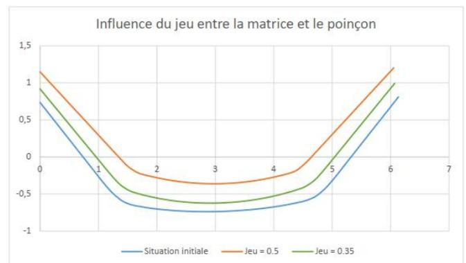
**Fig.5:** Sheet metal deformed after elastic springback for different gap between the sheet metal and the punch
