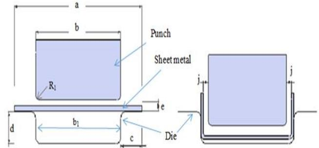
The dimensions of the characteristic sizes of the process illustrated in figure 1 are as follows:  $a=15$  cm,  $b=10-j$  (cm)  $c=2.5$ cm,  $d=1.5$  cm. The corner radius are  $R_1= 3$ mm (die and punch rounding radius are identical). The radius  $R_1$  and gap  $j$  will be the main variables in these simulations. The die and the punch will be considered as non-deformable solids in this study.
