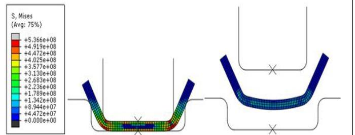
**Fig.4:** Stress fields for a 0.5mm gap between the sheet metal and the punch (Stress in Pascal). (a) Stress mapping during maximum deep-drawing, (b) deformation of the sheet metal after the deep-drawing operation
